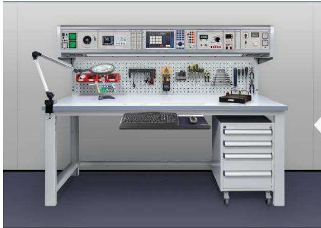
Picture of Electrical Test Bench, Input: 380~440V AC, 50/60 Hz, OUTPUT: 0~450V AC (VARIABLE) & 0~500V DC (Only for information purpose and may differ from actual products)
